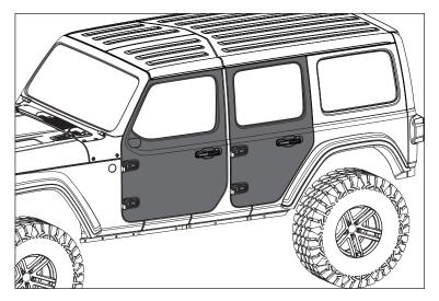
2. Loosely install Hinge Pins on Tube Doors using supplied M8 hardware.
