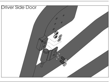
3. Using caution, slowly insert Tube Door in door hinges and reinstall factory door nuts.
