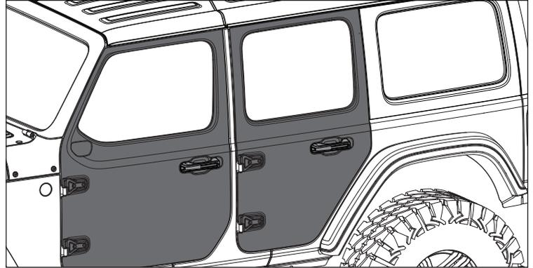
2. Loosely install Hinge Pins on Tube Doors using supplied M8 hardware.
