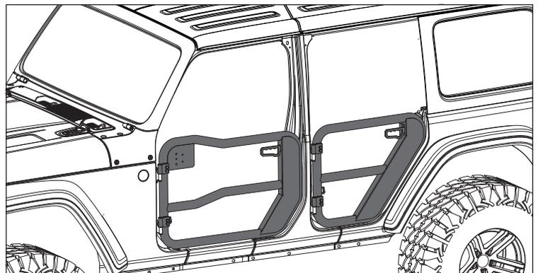
4. Close Tube Door and tighten Hinge Pin hardware. Install Check Strap and cycle Tube Door open and closed to ensure Hinge Pins are properly aligned and fully seated in door hinge.
