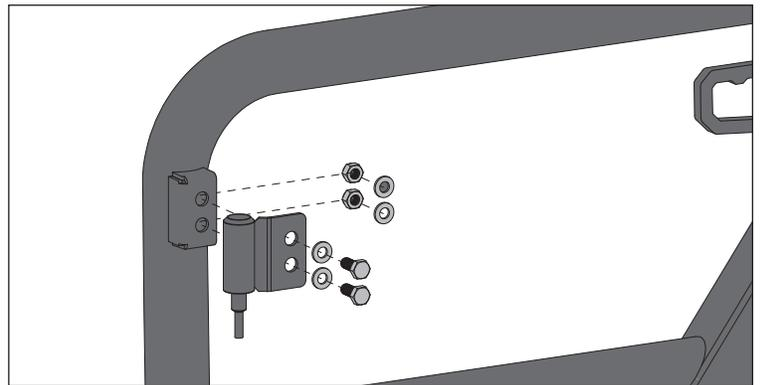
3. Using caution, slowly insert Tube Door in door hinges and reinstall factory door nuts.
