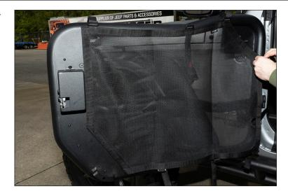
5. Secure Mesh Cover by looping straps around tube. DO NOT fully tighten at this time.
