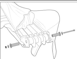
Replace the assembly pieces and tighten with a 13mm spanner and 6mm allen key.
