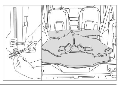
5. Unfold and attach hook strip to top of folded rear seat carpet. Align edges and anchor windows.
