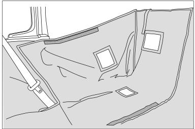
10. Loop straps around driver and passenger headrest to secure top portion of Cargo Cover upright.
